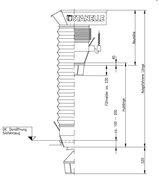
An immersion depth of the top cone into the opening of 150-200 mm needs to be calculated when calibrating the lift or the total length. During the loading process silo vehicles can be lowered for 100 mm, due to the additional weight. Notice
