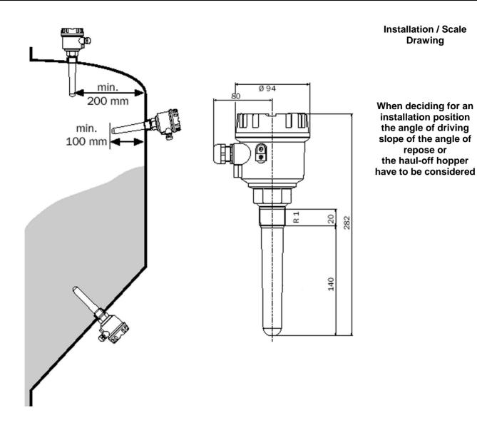
The limit level detection is used within silos with bulk materials. The silos can be made of various materials (e.g. metal, plastic, concrete), because this does not affect the metering process.
