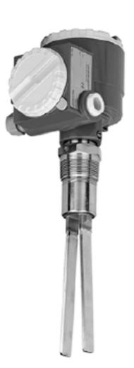
This vibration limit switch is a robust fill level sensor for silos with grained or dusty bulk materials, even if they have a very low piled weight. The different construction designs allow various areas of application, also in dangerous dust explosion areas of the zone 20 or in foodstuffs.
