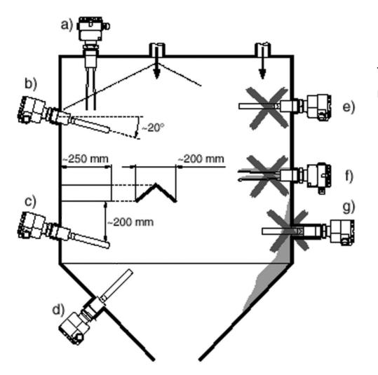
The vibration limit switch may be installed in any position according to the left side of the drawing.
