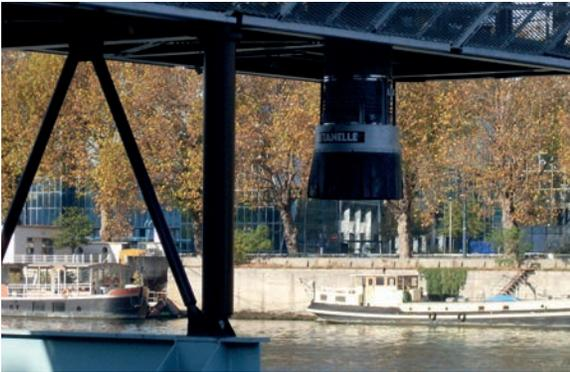
The Stanelle JET loaders TYPE **RONDO 350 / 400 / 500** with an extended hub are designed for loading ships and slagheaps. The required volume of exhaust air of approx. 2,000 - 3,000m<sup>3</sup>/h can be extracted via the suction nozzles by using an appropriate dedusting unit.
