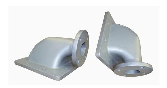
The gas-dust mixture is deflected at right angles through the silo inlet bend and introduced into the silo. Due to the space-saving design and use of the block flange, the conveying line can be guided close to the silo. This results in a favourable transport mass for assembled conveying lines. Weld-in or flanged flanges allow favourable installation options and trouble-free position adjustment during assembly.
