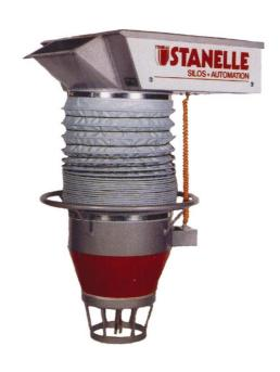
The Stanelle JET-LOADER TYPE JBM 220 QUADRO is designed for the loading of silo vehicles and containers with free flowing, dry bulk materials. The wide range of applications includes the mining-, chemical- and pharmaceutical industries - even in the explosion-proof areas.
