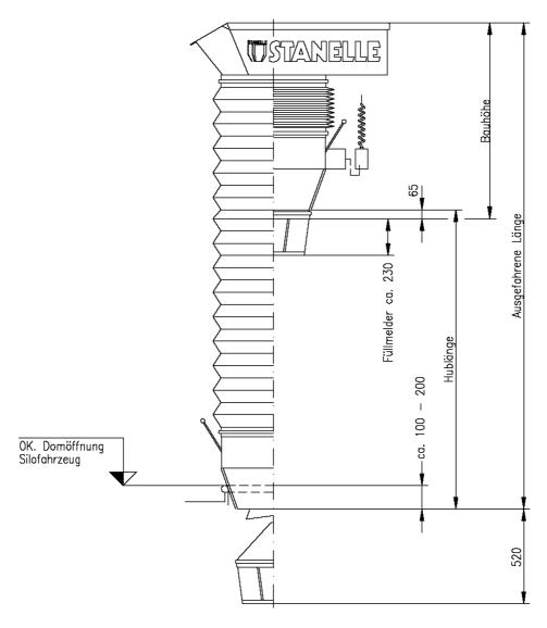
An immersion depth of the top cone into the opening of 150-200 mm needs to be calculated when calibrating the lift or the total length. During the loading process silo vehicles can be lowered for 100 mm, due to the additional weight.
