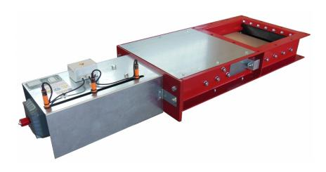
The **Flat slide gate TYPE SMFS GK Serie** will be mounted at the outlet of a silo or buffers to interrupt the free flow of bulk products. It ensures the best tightness of storaging of grainy bulk products with a grain size up to 50 mm.
